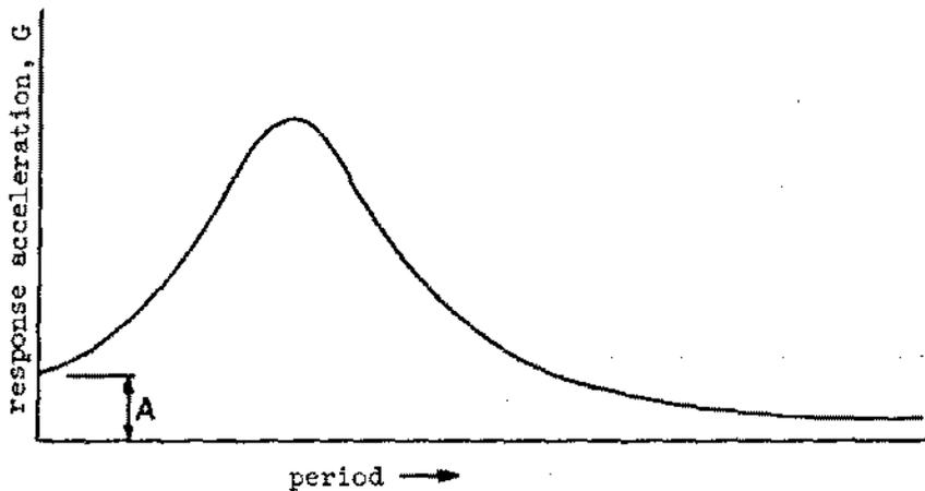
Figure 7 Typical Seismic Response Spectra
