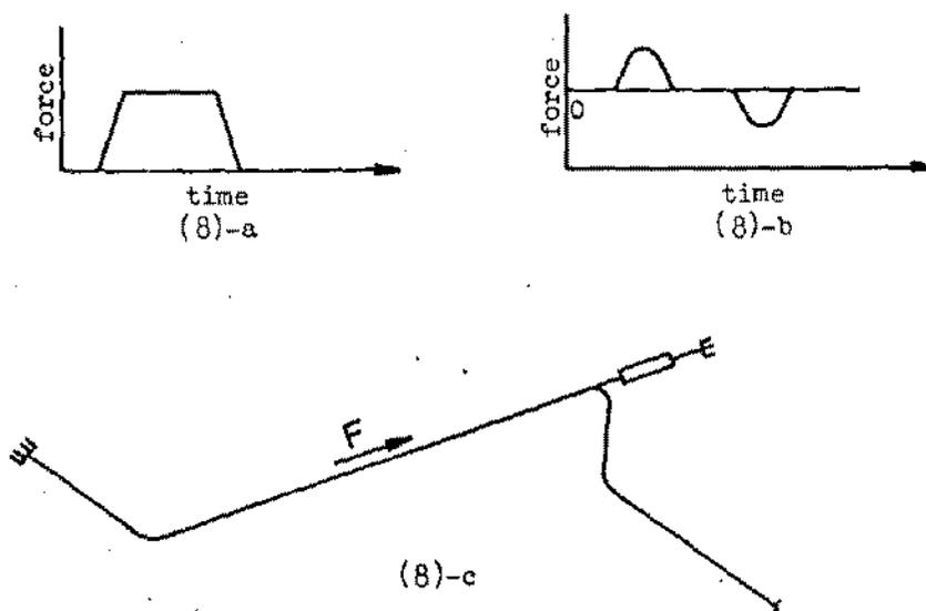
Figure 8 Typical Safety or Relief Valve Blowdown Forces
