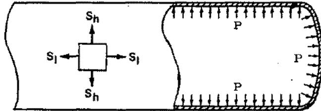
Figure 1. Pressure Loading
