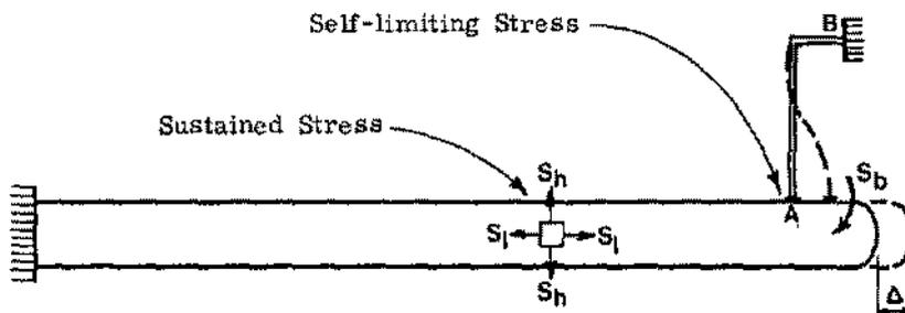
Figure 4. Stresses Caused by Internal Pressure
