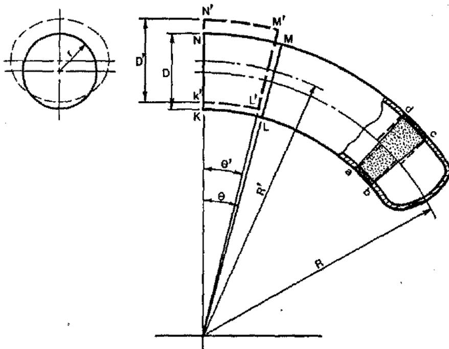
Figure 3. Pressurization of Bends
